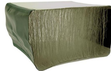
Figure 9: Drop-Stitch material cross-section showing internal drop yarns between the top and bottom layers. Drop yarns range from 1.3 to 8 inches.
