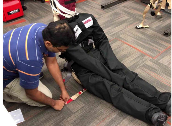
Figure 21: Lower to supine by releasing diagonal cords. ATD is stabilized in the AirLift and a flap on the AirLift is pulled out to give access to the cord release and inflation lanyard.
